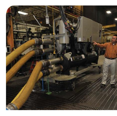
The tolerance for tons, kW/ton, and heat balance varies based on the chiller load and the operating conditions of the system. The specific tolerances for the test are listed on the test target sheet.
