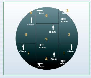
To determine the circular edge cut profile, which is located around the completed body section of dome end – mark the Armaflex circular edge with White marking chalk.
