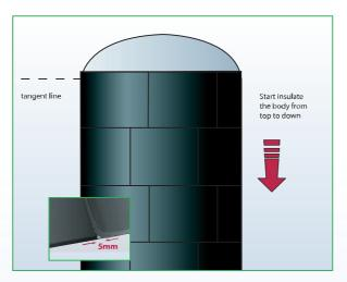
Install the Armaflex sheet panels from the domed end section of the vessel as shown. Use all-over adhesive coverage to both surfaces.
